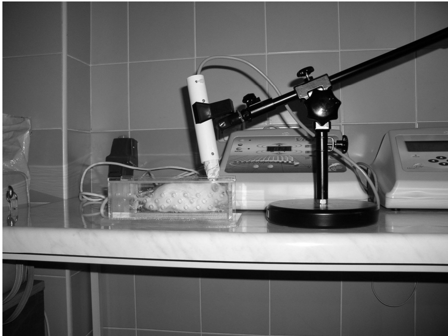
Fig. 1. Experimental system for simultaneous exposure of rat's head to and laser radiation and variable magnetic field generated by magneto-laser applicator of Viofor JPS device (Med & Life, Poland)
